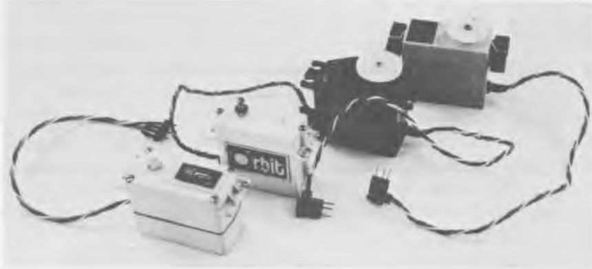
FIGURE 5-1 Model airplane servo of the type used in this project.
