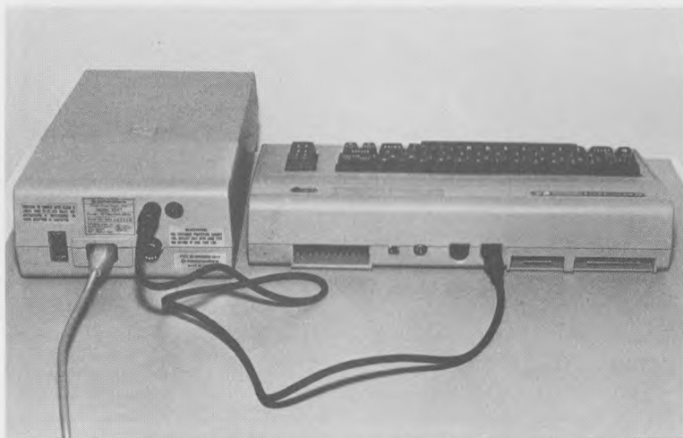
The 64 easily connects to the model 1541 disk drive via a single cable.
