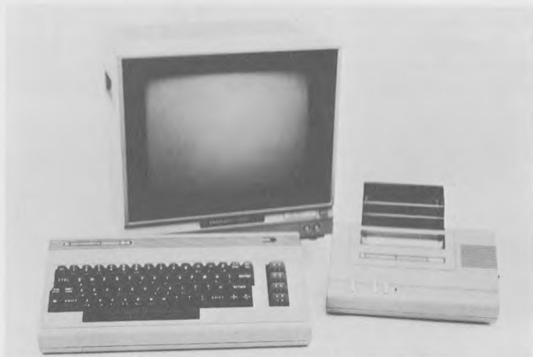
The Commodore 64 with the Commodore model 1701 color monitor and an 80-column graphics Plotter Printer.
