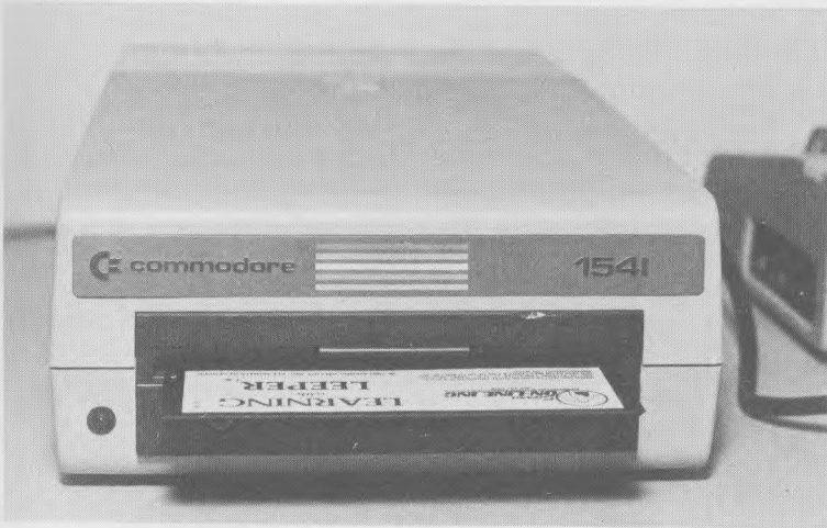
The model 1541 external 5¼-inch floppy diskette recorder and player offers high-speed and increased capacity for storing or playing back programs and data.
