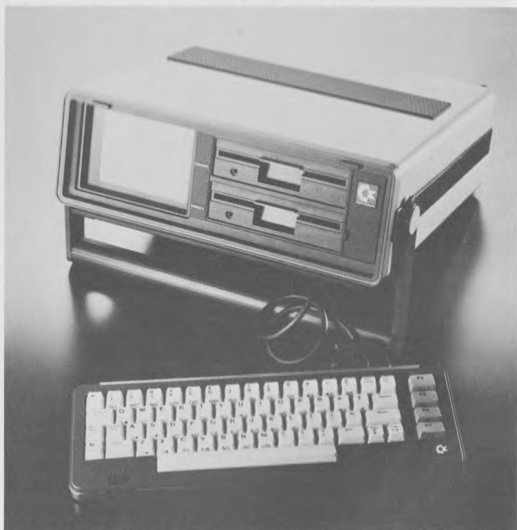
The Commodore 64's potent portable version has a 6-inch color monitor and a built-in single-disk drive. Called the Executive 64, it is slated for release in 1984.
