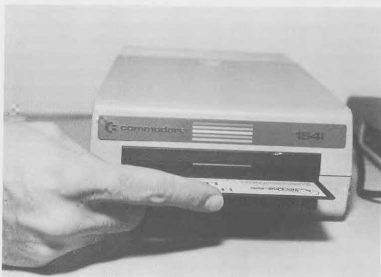
Inserting a disk into the model 1541 disk drive (label up, the oblong "reading" slot forward).
